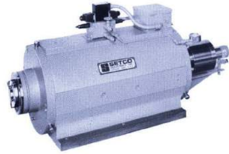
Photo #4051 Type 6250-36/18MLC-PD Two Speed Heavy Duty Motorized Milling Spindle rated 50/25 H.P. at 3600/1800 R.P.M. and arranged for continuous duty with constant torque. Milling spindle includes bayonet type power draw bar assembly and vari-load adjustable preload bearings.
