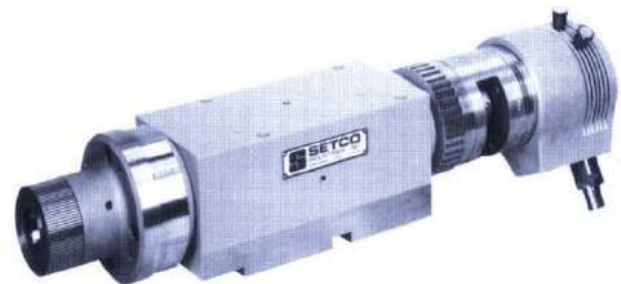
Photo #4015 Type 4305BY Boring Spindle Assembly arranged with an A2 6" Lathe Nose, 1.56" hole through arbor for coolant flow, SMW chuck assembly and high speed rotary jet cylinder, special pulley/cylinder adapter and draw tube for feeding 1" diameter stock.
