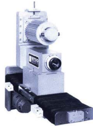
Photo #4048 Type 4303M Milling Spindle with universal 'Kwik-Switch' nose and integral motor mounting arrangement with a 2:1 ratio drive and servo motor. Spindle mounted to riser block and 8" wide dovetail slide with ball screw and servo drive package.
