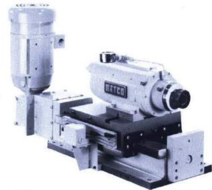
Photo #4103 This precision spindle/slide assembly consists of a motorized Size 6 milling spindle rated 2 H.P. at 3600 R.P.M. with universal 'Kwik-Switch' nose. Spindle is precision keyed and aligned to a Type SHL12FGD, 12" wide, Hardened Steel Way Slide equipped with precision ground ball screw and double preloaded ball nut which is directly coupled to a motor with right angle gear box.
