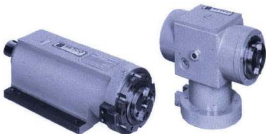
Photo #3992 Type 4206B-Y Precision Foot Mounted Boring Spindle Assembly arranged with a special nose construction to adapt a Type 2RA-Y Right Angle Milling Head with a #40 NMTB nose.
