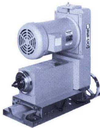
Photo #4080 Precision milling spindle/slide assembly consisting of a 4304M Spindle with #40 NMTB nose and integral motor mounting bracket/belt guard, drive system which is mounted to a manual 10" wide dovetail slide assembly.
