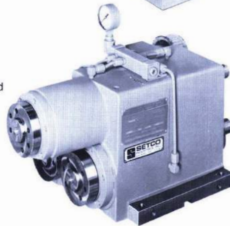
Photo #3647 Type 7CB05G Super Precision Seven Cluster Geared Spindle System includes intermediate drive package, heating sensors for temperature control, adjusting blocks and fitting spacers, precision integral gear box with single input shaft offering individual speeds at each spindle and lube pump all mounted on one sub-plate assembly.
