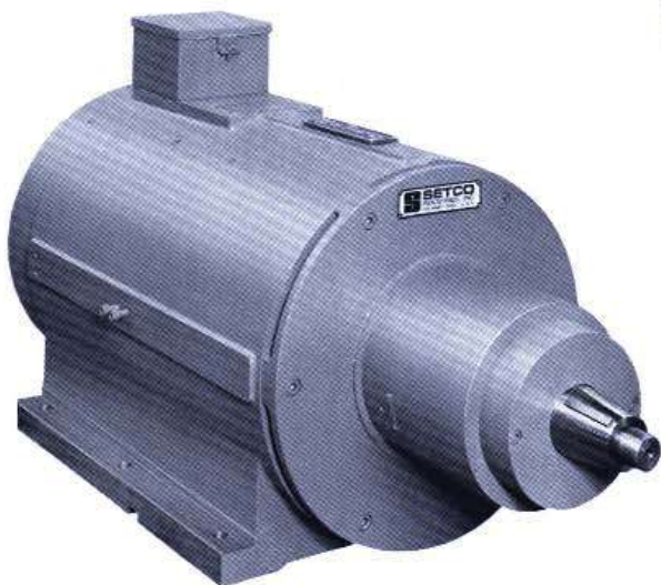
Photo #3790 Type 6150-18G fan cooled 50 H.P. at 1800 R.P.M. Motorized Grinding Spindle with external taper nose.
