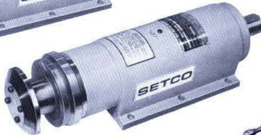
Photo #3254 Type 4205GY Foot Mounted Grinding Spindle arranged for 5000 R.P.M. with oil mist lubrication and Type 7A Wheel Holder.
